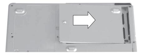
**4** Slide the battery lock to the locked position.
